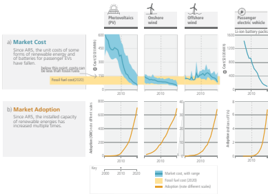
Figure 2.4: Unit cost reductions and use in some rapidly changing mitigation technologies. The top panel (a) shows global costs per unit of energy (USD per MWh) for some rapidly changing mitigation technologies. Solid blue lines indicate average unit cost in each year. Light blue shaded areas show the range between the 50th and 95th percentiles in each year. Yellow shading indicates the range of unit costs for new fossil fuel (coal and gas) power in 2020 (corresponding to USD 55 to 148 per MWh). In 2020, the levelized costs of energy (LCOE) of the three renewable energy technologies could compete with fossil fuels in many places. For batteries, costs shown are for 1 MWh of battery storage capacity; for the others, costs are LCOE, which includes installation, capital, operations, and maintenance costs per MWh of electricity produced. The literature uses LCOE because it allows consistent comparisons of cost trends across a diverse set of energy technologies to be made. However, it does not include the costs of grid integration or climate impacts. Further, LCOE does not take into account other environmental and social externalities that may modify the overall (monetary and non-monetary) costs of technologies and alter their deployment. The bottom panel (b) shows cumulative global adoption for each technology, in GW of installed capacity for renewable energy and in millions of vehicles for battery-electric vehicles. A vertical dashed line is placed in 2010 to indicate the change over the past decade. The electricity production share reflects different capacity factors; for example, for the same amount of installed capacity, wind produces about twice as much electricity as solar PV. Renewable energy and battery technologies were selected as illustrative examples because they have recently shown rapid changes in costs and adoption, and because consistent data are available. Other mitigation options assessed in the WGII report are not included as they do not meet these criteria. (WGII Figure SPM.3, WGII 2.5, 6.4)
